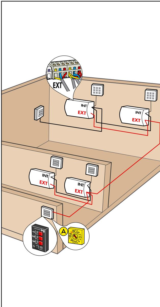
**English:** Several groups can be connected using the WLL 100 cable set, so that all motors can be operated from one central keypad. Connect the central keypad to the "EXT" outlet of one of the control units and set the code switch in the keypad to the position "A". Up to 32 control units can be connected in series.
