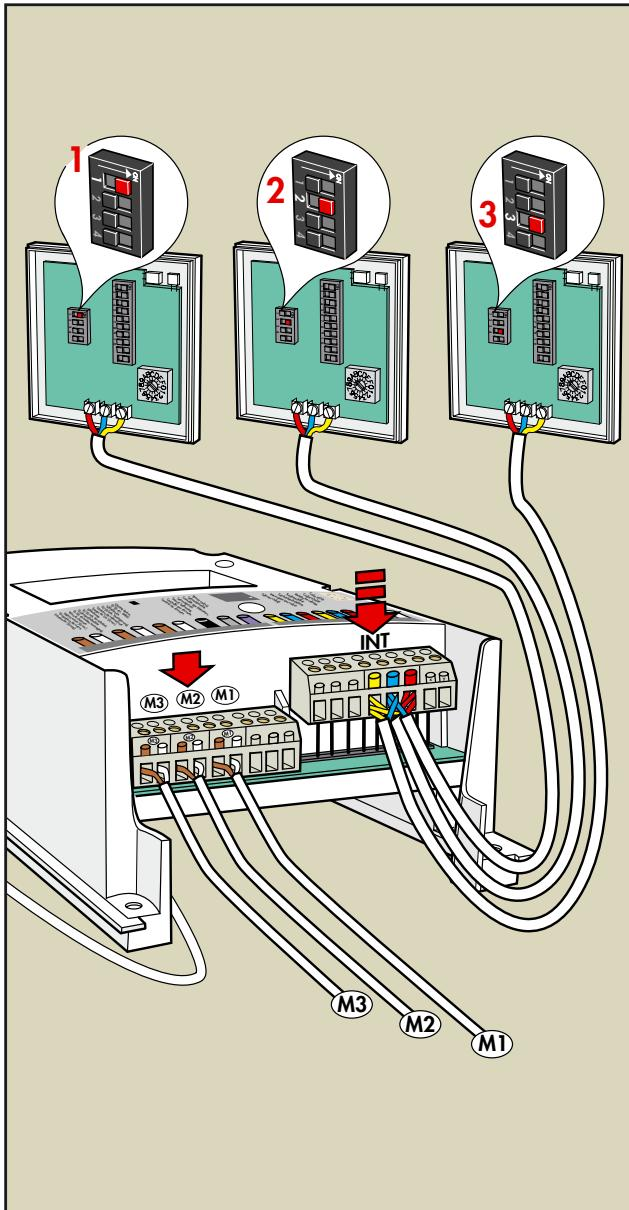
**English:** Three motors can be operated individually from three separate keypads. Connect keypad cables to outlet "INT" of the control unit. Set the switch to the same number as the motor which is to be operated to the "ON" position.
