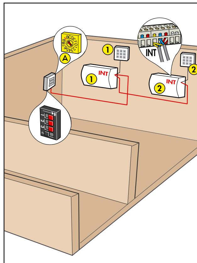
**English:** Control units can be linked in series using the WLL 100 cable set. Motors can then be operated from local keypads (1 + 2) and/or master keypad (A). MASTER WLI 110: Connect to outlet "INT" of control unit. Set switches 1, 2 and 3 to "ON" position. MASTER WLI 130: Connect to outlet "INT" of control unit. CODE SWITCHES: Set master keypad to "A". Local keypad and control unit code switches must have identical settings. Up to 32 control units can be connected in series.
