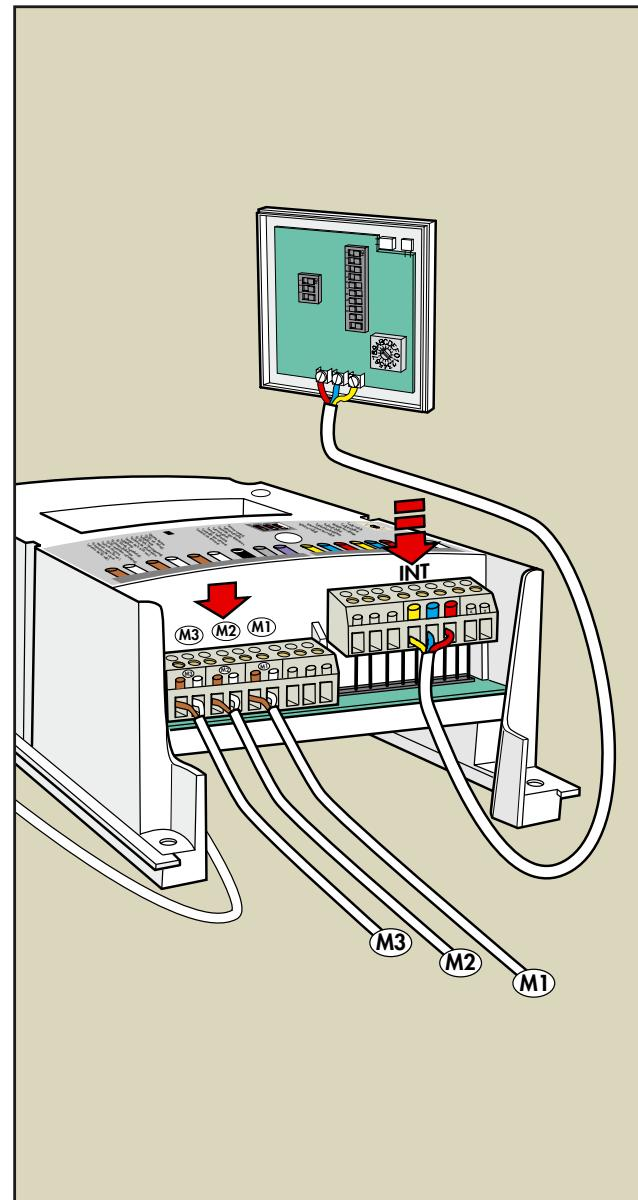
**English:** Three motors can be operated individually from one keypad. The keypad has three rows of buttons; each row operates one motor.
