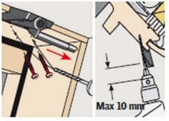
ENGLISH: Determine measurement X on the top frame and fit drilling jig temporarily.
