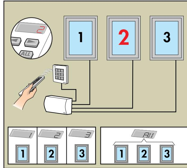
**English: Individual operation:** Select the window to be operated (in the example window number 2 has been selected) by activating  $\blacktriangle/\triangledown$ . Operate the window by pressing  $\blacktriangle$  or  $\triangledown$ .
