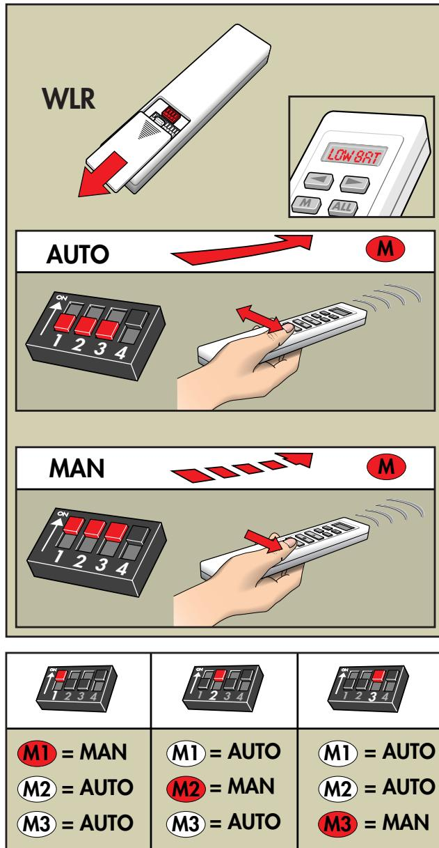
**English:** If a switch (1, 2 or 3) is set in position "AUTO" (automatic), the corresponding motor will travel to the end-stop after one press of the button. If a switch is set in position "MAN" (manual), the motor will run only as long as the button is pressed (recommended for electrically operated Venetian blind). "AUTO/MAN" can be set individually for each motor. The examples at the bottom of page 7 show which switch belongs to which motor.
