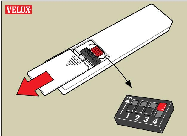
**English:** When operating up to three motors per window, set switch 4 in position "ON".
