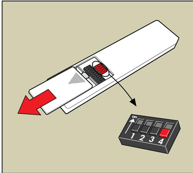
**English:** When operating one motor per window, set switch 4 in position "OFF".
