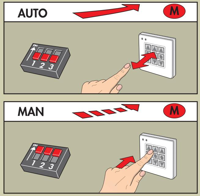
**English:** If a switch (1, 2 or 3) is set in position "AUTO" (automatic), the corresponding motor will travel to the end-stop after one press of the button. If a switch is set in position "MAN" (manual), the motor will run only as long as the button is pressed (recommended for electrical Venetian blind). "AUTO/MAN" can be set individually for each motor. The examples at the bottom of page 7 show which switch belongs to which motor.
