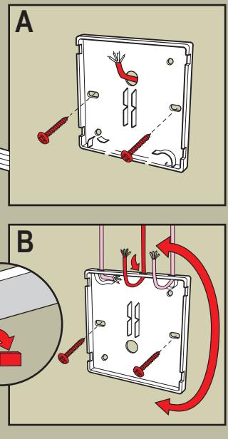
**English:** Fit keypad WLI 130 on wall. **Hidden wiring (A):** Run cable through hole in back plate. **Visible wiring (B):** Decide where to lead the cable through. Make hole in side of back plate by removing knock-out. Rotate back plate 180° if the cable is to be led through at top of the keypad.
