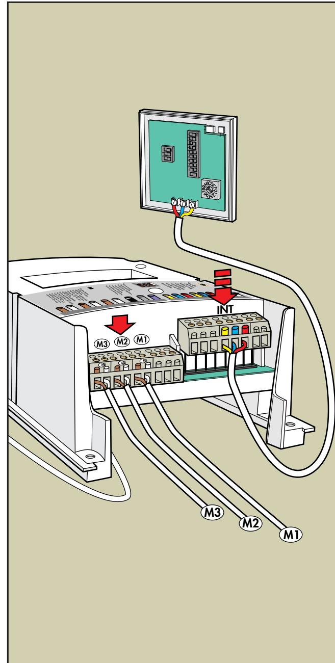
**English:** Three motors can be operated individually from one keypad. The keypad has three rows of buttons; each row operates one motor.
