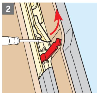
**ENGLISH: Disengage springs:** Open window, pull sash slightly downwards and insert red plastic clips **1**. Push sash upwards and disengage hooks **2**.
