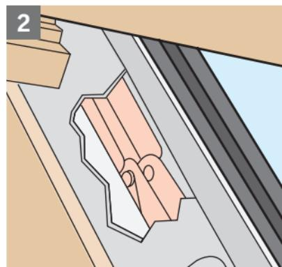
**ENGLISH: Connection of springs with fittings:** Push sash upwards, ensuring that fittings and springs on both sides automatically connect **1, 2**.
