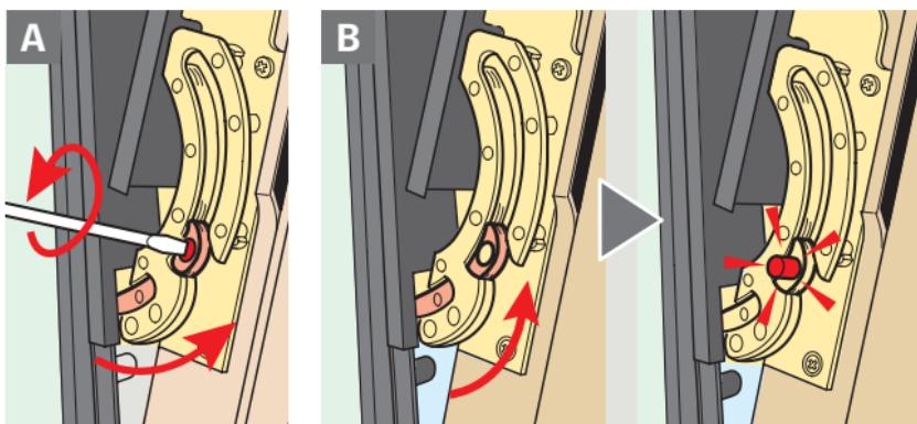
**English:** Replace window sash. The push button is automatically released, when the window is closed **A , B**.
