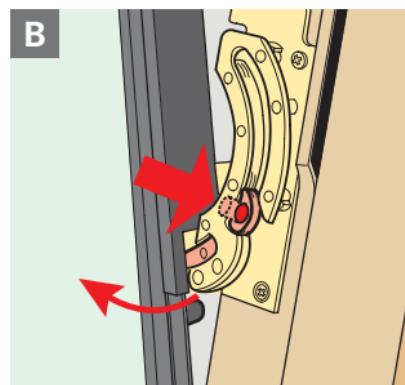
**ENGLISH:** Remove window sash. Hinges may either have a screw **A** or a push button **B**. Press in push button, eg with a screwdriver.
