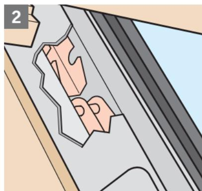
**ENGLISH: Disengage springs:** Open window. Push sash upwards and tip up sliding devices **1** , **2** .
