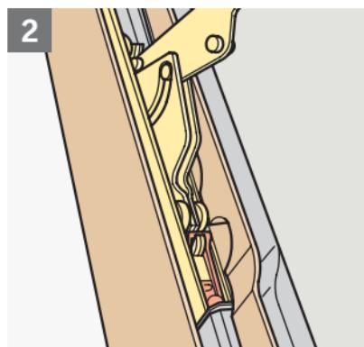
**ENGLISH:** Push sash upwards, while pulling fittings downwards to connect with springs on both sides **1 , 2**.
