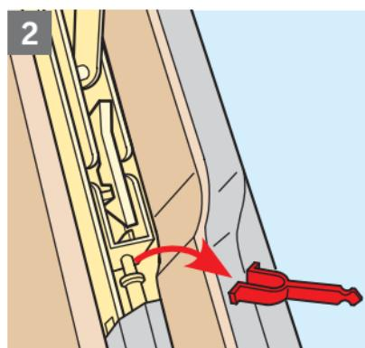
**ENGLISH: Connection of springs with fittings:** Push sash upwards, ensuring that fittings and springs on both sides automatically connect 1. Then pull sash slightly downwards to remove red plastic clips 2.
